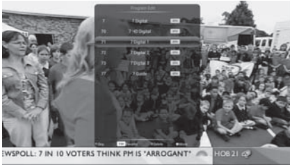
Program Edit: Click to enter the submenu, there are three shortcuts, by pressing ▼ / ▲ to select the channel you want to operate, you can jump the selected channel, rename the channel, and increase or delete the channel to the favorite program list operating.
