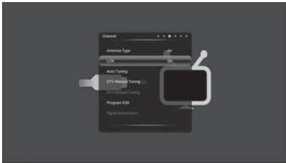
LCN: Whether to open the logical channel number sort.
