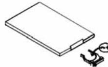
3. Insert the Battery Holder into the Remote Control.
