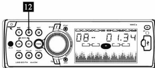
2. During playback, press „2 INT” button, one of the number button 12 to play the first 10 seconds of each track from USB/SD MMC, the Display will show „INT, track number and elapsed time” (see the picture), which indicates INT functions already activated.
